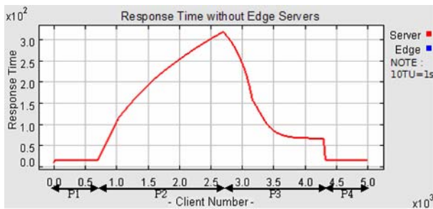
Fig. 4. Response time per client without Edge server
